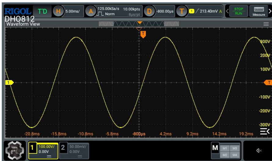
Figure 4: Reconstructed 60Hz clean output waveform.
