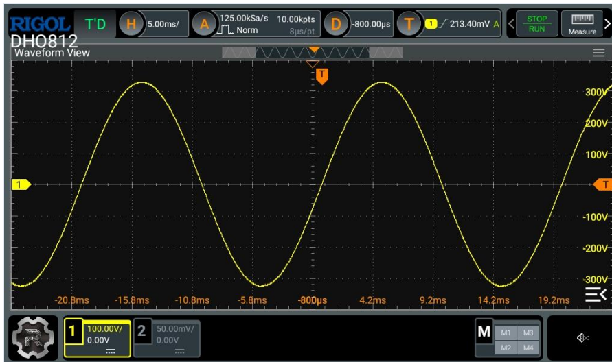
Figure 3: Reconstructed 50Hz output waveform from the RPS series, displaying a smooth, symmetrical sine wave.
