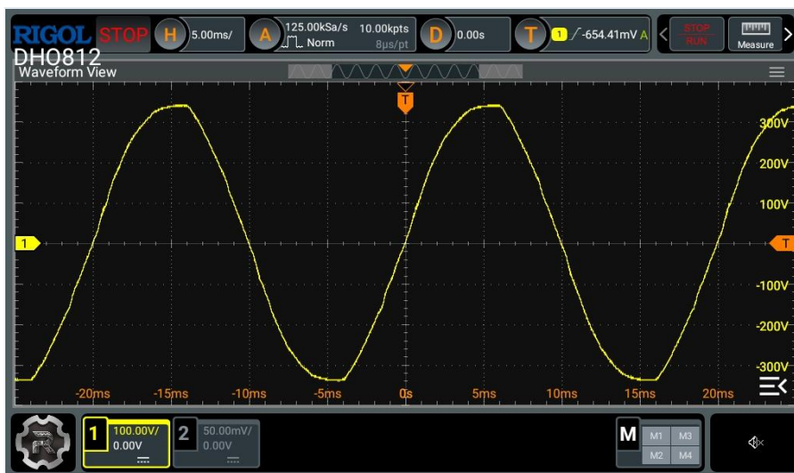
Figure 1: Distorted incoming 50Hz mains supply waveform captured via laboratory oscilloscope.
